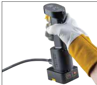
Fig. 20 Using the nVent ERICO Cadweld Plus Impulse Exothermic Welding Control Unit, lift the trigger cover and press the ignition button and hold. You will see the 6 lights on the top of the control unit light up as it is charging. After the 6th light is illuminated, the control unit will send a charge to the ignition strip, initiating the Cadweld Plus exothermic reaction.
