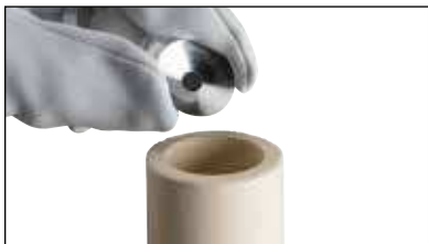
Fig. 8 Place the steel disk into the Cadweld One Shot with the concave side facing up.
