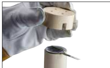
Fig. 10 Place the ceramic lid onto the mold.
