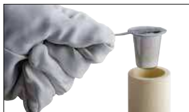
Fig. 9 Place the welding material cup into the top of the mold. Make sure the ignition strip nests into the recess on the top edge.
