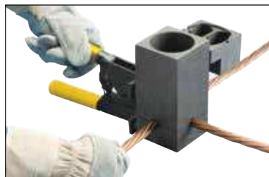
Fig. 13 Insert the conductors and position them for the connection.
