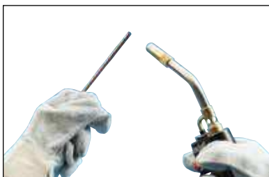
Fig. 4 The conductors should be clean and dry before the connection is made. Use a propane torch to dry wire conductors and remove remaining cleaning residue, solvent, or water before making the Cadweld connection.
