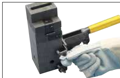
Fig. 7 Tighten the clamp thumbscrews onto the mold.
