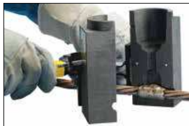
Fig. 28 Open the mold and remove the connection. Use care to prevent chipping the mold. Avoid contact with hot materials. See the "Cadweld Quality Standards" section to see whether a quality connection has been made.
