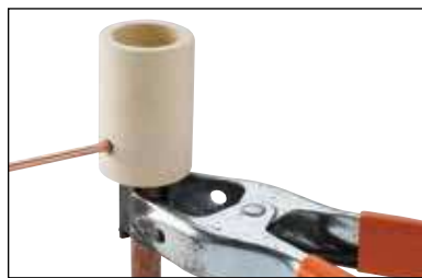
Fig. 7 Insert the conductors and position them for the connection. To support the One Shot on the rod, use locking pliers or clamp B399P (sold separately).
