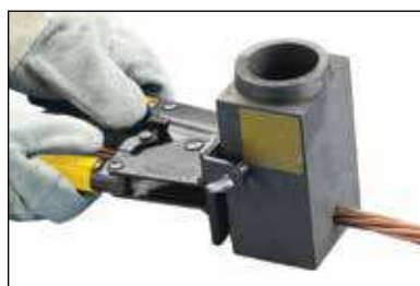
Fig. 16 Close the clamp tightly once the conductors are properly positioned.
