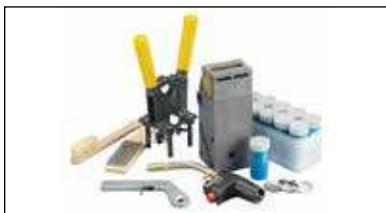
Fig. 2 Gather the proper materials and equipment for the type of connection you are making. The typical Cadweld system requires a graphite mold, handle clamp, welding material, natural bristle brush for mold cleaning, wire brush for cleaning/preparing conductors, flint igniter, and propane torch.
