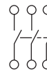
Fig. D MHU361, MHU362, MHU363, MHU364, MHU361R, MHU362R, MHU363R, MHU364R 3 pole, 3 wire
