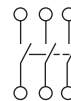
Fig. D MHU361, MHU362, MHU363, MHU364, MHU361R, MHU362R, MHU363R, MHU364R 3 pole, 3 wire
