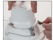
Rotate the three side clips into place to secure the trim to the LED light module. Ensure all three clips are securely engaged.
