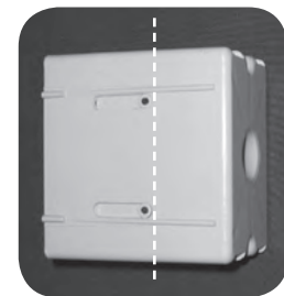
Slider plate retracted sets box in fully adjusted forward position for maximum wall substrate thickness of 1-3/8".
