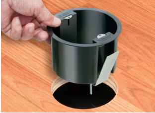
1 Cut a 5" diameter opening. Insert box.
