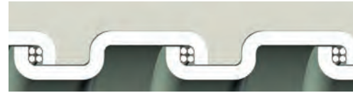
Square-Locked Design with cord packing 5/16" through 1-1/4"
