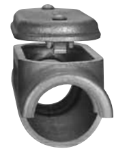
Crouse-Hinds Form 7 (C57, 1-1/2") 26 Cubic Inches Capacity
