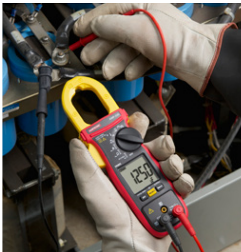
AMP-320 AC/DC Clamp Meter Electrical Motor Maintenance
