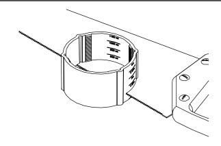
Pull wires to the box (see chart below for wiring capacity for each cover). Re-insert the concrete cap to prevent damage to the box until the cover is ready to be installed.
