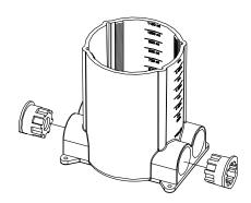
Position box and secure to prevent floating during the concrete pour (Orientation of the receptacle is aligned with the conduit). For above grade, screw or nail the box to the concrete form. For on-grade applications, drive rebar next to the box and secure with wire.
