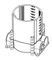
Cut the conduit to length and cement to ports or reducers. Install concrete cap and pour concrete to desired depth using the graduated markings on the box exterior as a guide.
