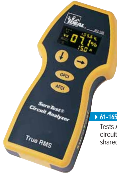
Troubleshoots branch circuit problems with a variety of tests at the receptacle.
