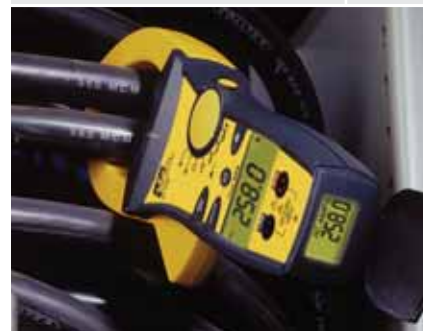
Large jaws for clamping around multiple conductors
