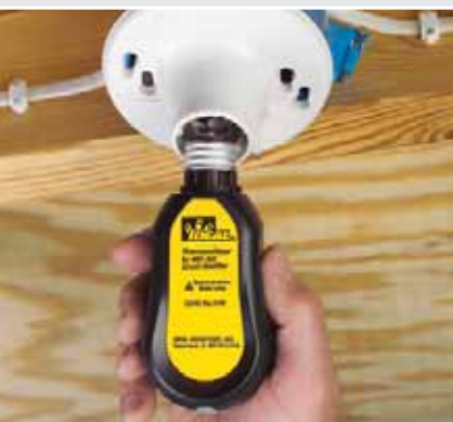
Lighting adapter allows connection to light fixtures
