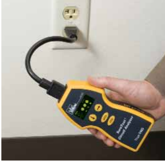
Troubleshoots branch circuit problems with a variety of tests at the receptacle.
