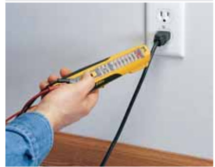
Non-contact voltage sensor easily locates breaks in power cords.
