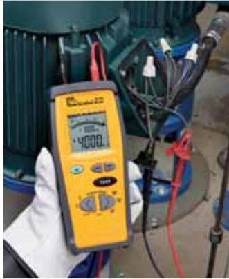
Tests insulation on motor windings
