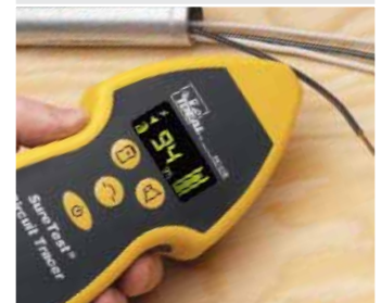
Individual wires can be sorted, opens can be located and shorts can be isolated.
