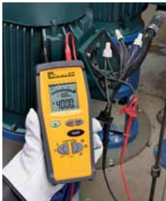
Tests insulation on motor windings
