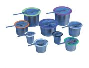
nVent ERICO Cadweld Plus Welding Material, F20, allows for an expedited, permanent grounding connection using premeasured, self-contained cups. Each package of welding material can be easily placed into the mold and safely ignited with the nVent ERICO Cadweld Plus Impulse Exothermic Welding Control Unit to create an irreversible bond.
